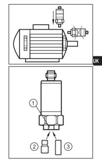
Tighten the unit with a tightening torque of 8 Nm.
